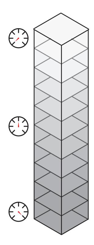
Then the total weight is 624 lbs. This weight is divided over 144 square inches. This gives us a pressure of 4.33 psi at the bottom of the 10 foot column of water.
